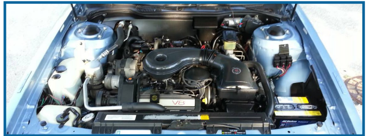
Engine: 4.5 liter - 273ci - 155 hp, V-8 (front wheel drive)
